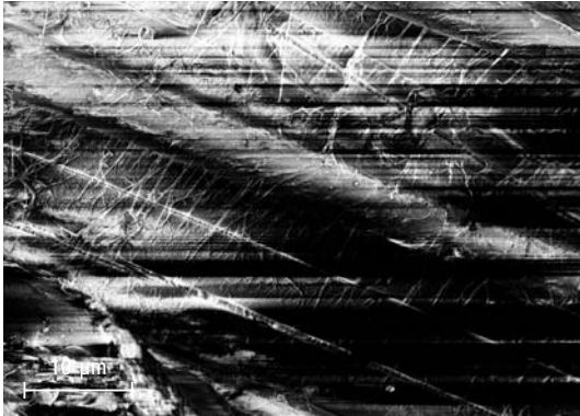
Fig. 4a: Uncoated, non-conductive glass fibers with epoxy imaged without using charge compensation. Chamber SE detector, 2 kV, WD 6 mm: strong image distortion.
