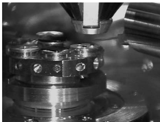
Fig. 1: TV image of the charge compensation system inserted into the chamber.
